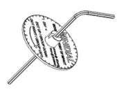
Thread hex 1.5mm wrench into minidial to gage adjustment as you turn.
