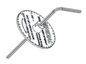
Thread hex wrench into minidial to gage adjustment as you turn.
