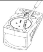
When removing the battery, always lever against the body not the terminals.
